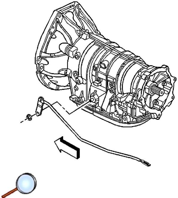
1. Install the shift control linkage to the vehicle.
